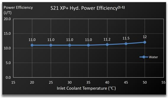
(3-1) The hashrate value, and power efficiency on wall are all typical values. The actual hashrate value fluctuates by  $\pm 3\%$ , and the actual power efficiency on wall fluctuate by  $\pm 5\%$ .
