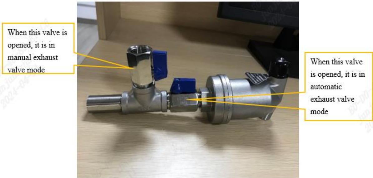
Figure 7-13 Cooling tower exhaust valve
