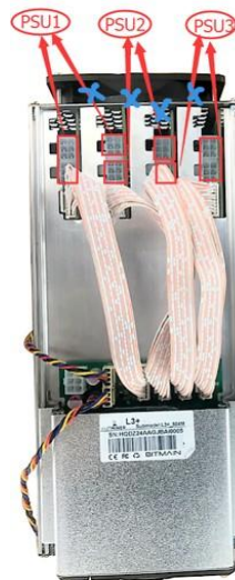
Figure 2-- 2. PCI-- E Connectors -- Incorrect Connection
