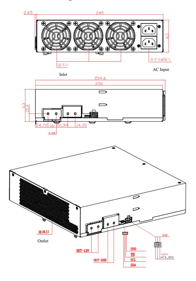
• Power supply distribution on the front panel: 2 zigzag AC input interfaces;
